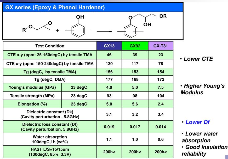
GX13:180deg.Cx90min curing, Others:190deg.Cx90min
