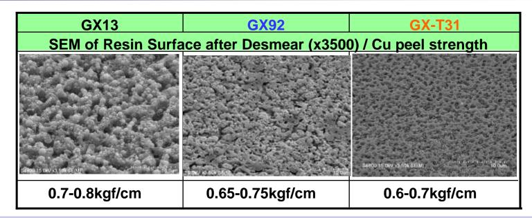
The key of fine line formation is to lower profile (smooth surface) with keeping high peel strength.
