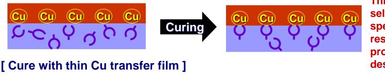
Thin Cu works for self-assembly of specific bonds on the resin surface and as a protective layer against desmear.
